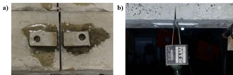
Figure 3: (a) Metal plates glued on the prismatic specimens; (b) extensometer placed on the prismatic specimens for three-point bending tests.
