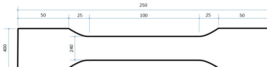
Figure 2: Specimen geometry used for tensile tests.
