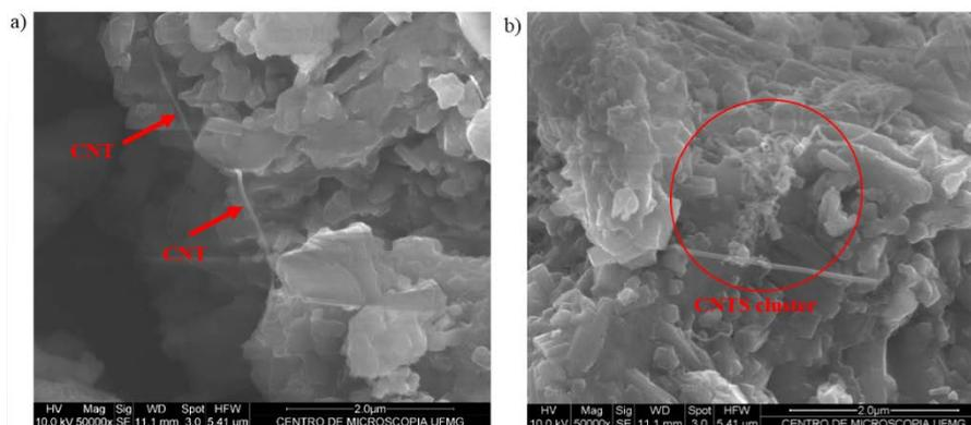
Figure 9: Scanning electron microscopy images of the anhydrous cement with (a) 0.05% of CNTs; (b) with 0.10% of CNTs
