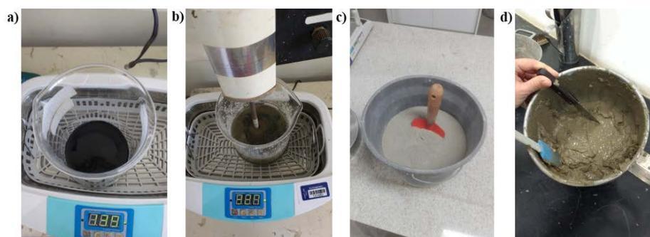
Figure 1: (a) Carbon nanotubes and isopropanol by sonication; (b) Carbon nanotubes, cement and isopropanol mixture being mechanically stirred and sonicated; (c) dry powder cement particles incorporated with CNTs mixed with the remaining quantity of cement; (d) cement paste with carbon nanotubes.
