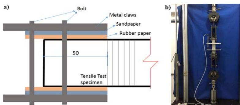
Figure 5: (a) Sketch showing the assembly and preparation of the specimens for tensile tests; (b) Specimens properly positioned in the equipment before testing
