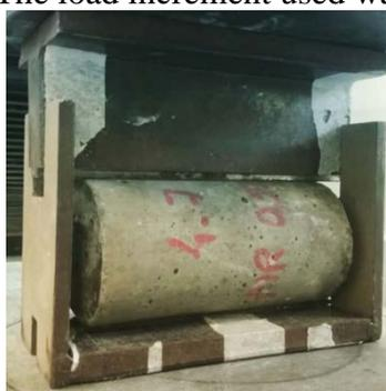
Figure 4: Splitting tensile strength test
